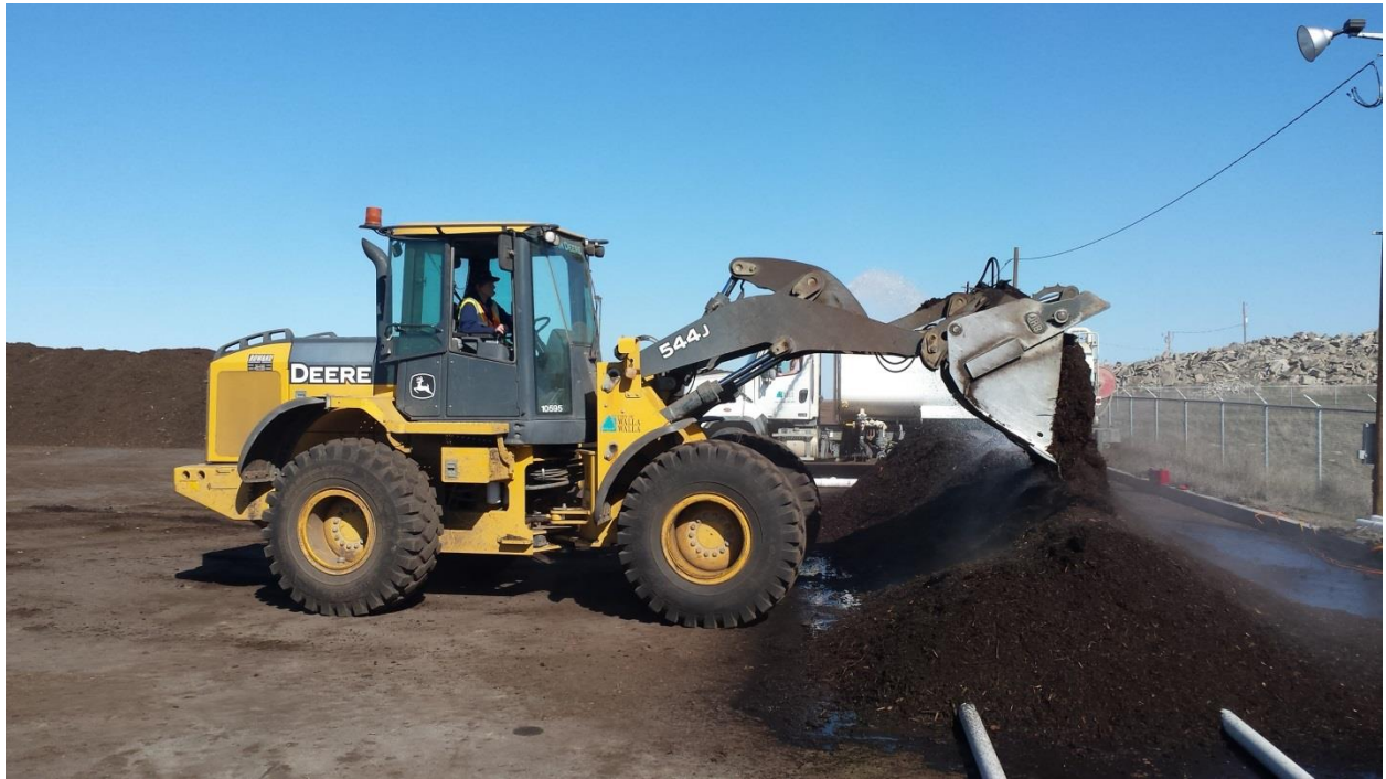
Placing Freshly Shredded Green Waste on Top of the Plenum Layer
