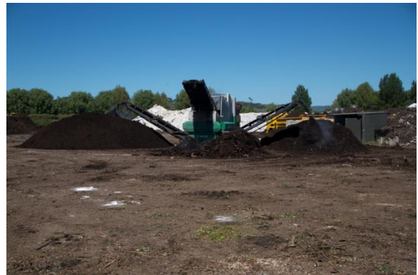
Photo 10: Star screen, dividing the compost into three size fractions.
